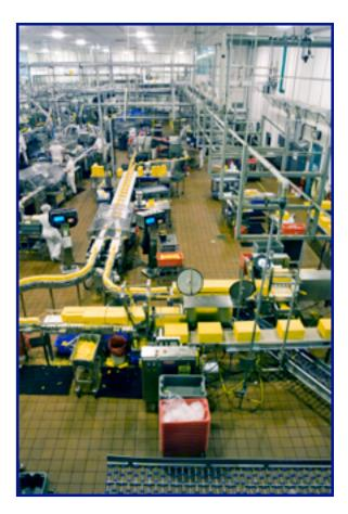
Nestlé has installed knowledge automation systems in real-time applications at their processing facilities. Real-time readings from a plant programmable controller are collected and provided to a knowledge automation system, which performs an analysis on the process status. Messages that guide the operator in optimizing the operations are then generated.
